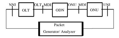
Figure 3-1—Test equipment configuration
