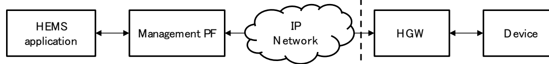
Outside the home (Internet) Inside the home (HN) Figure 3. HEMS based on HN service architecture
