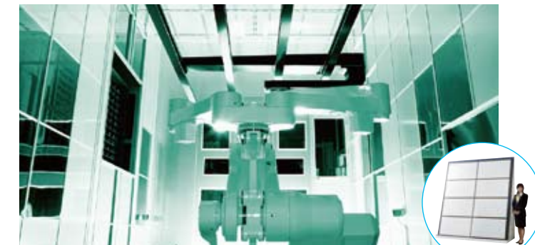
A robot moves a large 0.7-mm thick mother glass panel in an LCD factory.
